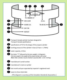
**Note:** Cylinder markings may be laid out differently on the collar than shown above.
