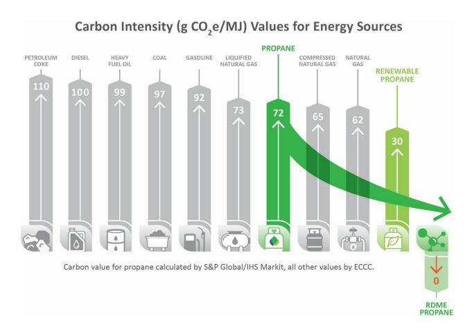
Renewable propane is already being produced in the U.S. and Europe. Unlike conventional propane, renewable propane can be made from a variety of renewable feedstocks. The most common form of renewable propane today is a byproduct of renewable diesel and sustainable aviation fuel made primarily from plant and vegetable oils, animal fats, or used cooking oil.
